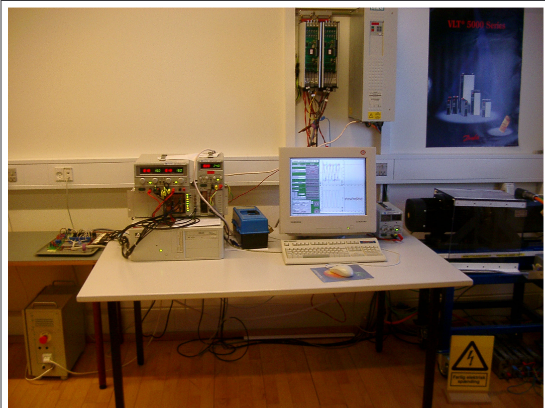
Figure 86 Complete test system with six-phase induction motor, 2x3-phase Danfoss VLT, measurement board and a D-Space control computer.
